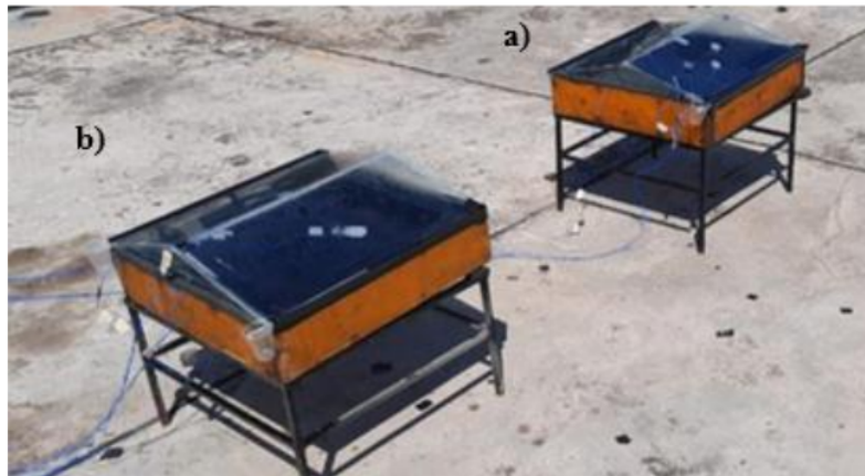
Figure 1. Solar distillation systems consisted of: a) Using flat absorber plate b) Using fin absorber plate with PCM storage
